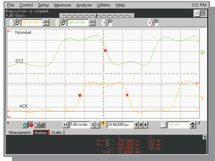
Figure A: Shows a peak-to-peak value of 503 mV for the ACK# signal with drive strength set to nominal
